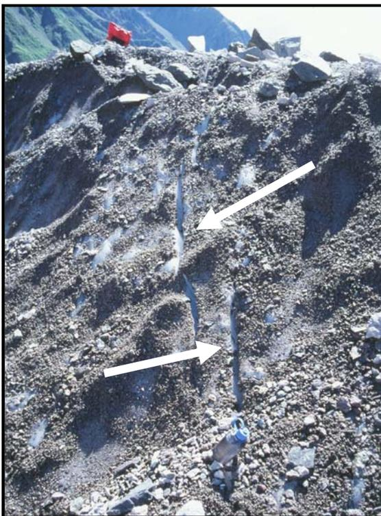
Figure 18. Photo showing fresh fractures that propagated through the drill site. The width of the fractures is approximately 4-7cm.
