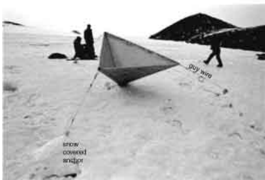
Figure 4.7: A trihedral corner reflector.
