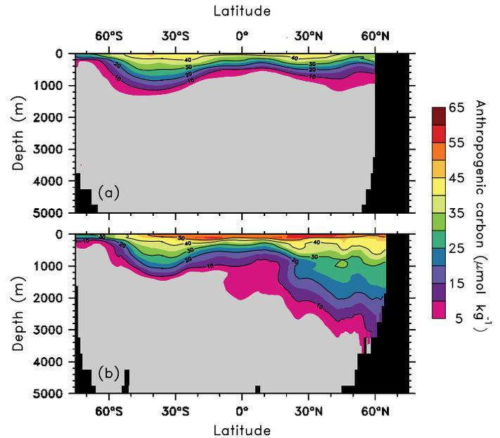
**Figure 5.11.** Mean concentration of anthropogenic carbon as of 1994 in  $\mu\text{mol kg}^{-1}$  from Sabine et al. (2004b) averaged over (a) the Pacific and Indian Oceans and (b) the Atlantic Ocean. The calculation of anthropogenic carbon is described in the caption of Figure 5.10 and in the text (Section 5.4).
