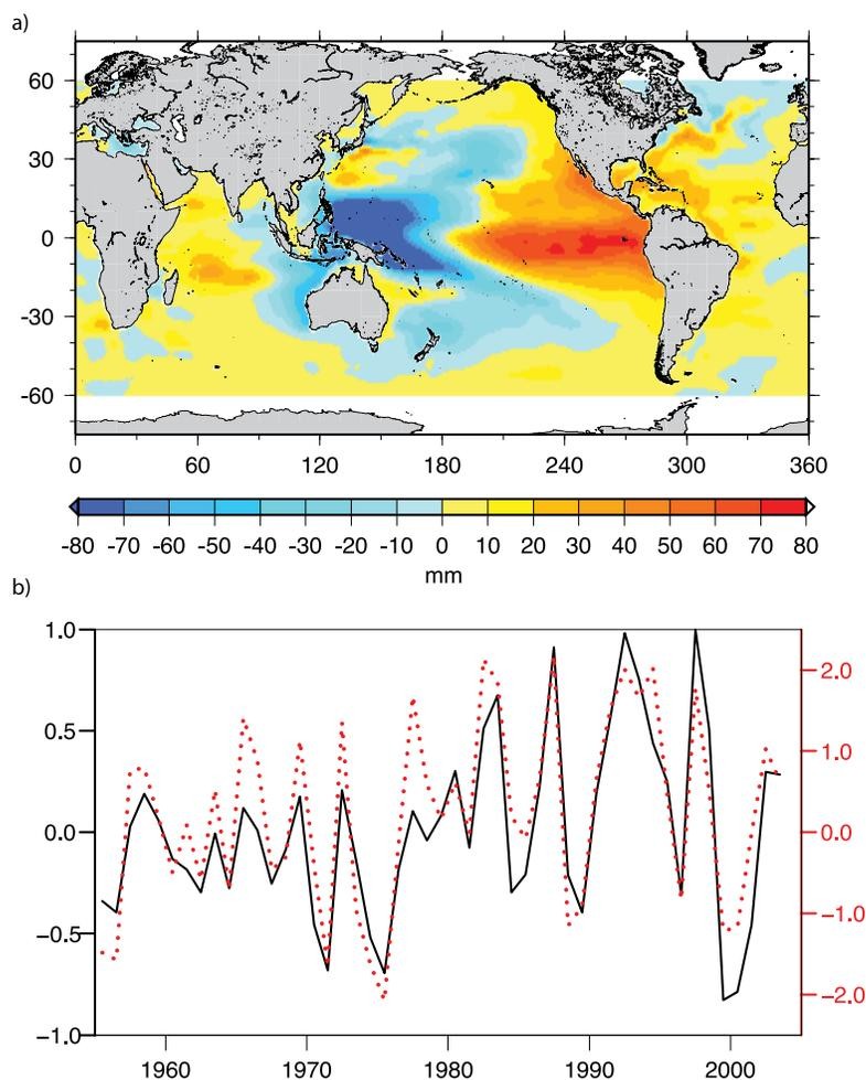
**Figure 5.20.** (a) First mode of the EOF decomposition of the gridded thermosteric sea level time series of yearly temperature data down to 700 m from Ishii et al. (2006). (b) The normalised principal component (black solid curve) is highly correlated with the negative Southern Oscillation Index (dotted red curve).
