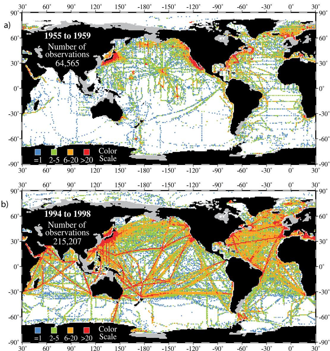
**Figure 5.A.1** The number of ocean temperature observations in each  $1^\circ$  grid box at 250 m depth for two periods: (a) 1955 to 1959, with a low density of observations, and (b) 1994 to 1998, with a high density of observations. A blue dot indicates a  $1^\circ$  grid box containing 1 observation, a green dot 2 to 5 observations, an orange dot 6 to 20 observations, and a red dot more than 20 observations.
