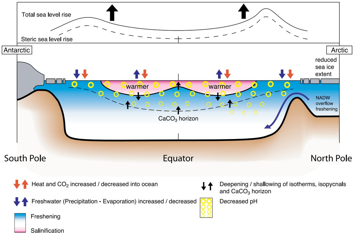
**Figure 5.23.** Schematic of the observed changes in the ocean state, including ocean temperature, ocean salinity, sea level, sea ice and biogeochemical cycles. The legend identifies the direction of the changes in these variables.
