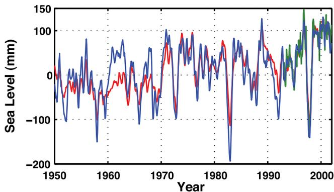
**Figure 5.18.** Monthly mean sea level curve for 1950 to 2000 at Kwajalein ( $8^{\circ}44'N$ ,  $167^{\circ}44'E$ ). The observed sea level (from tide gauge measurements) is in blue, the reconstructed sea level in red and the satellite altimetry record in green. Annual and semi-annual signals have been removed from each time series and the tide gauge data have been smoothed. The figure was drawn using techniques in Church et al. (2004) and Church and White (2006).
