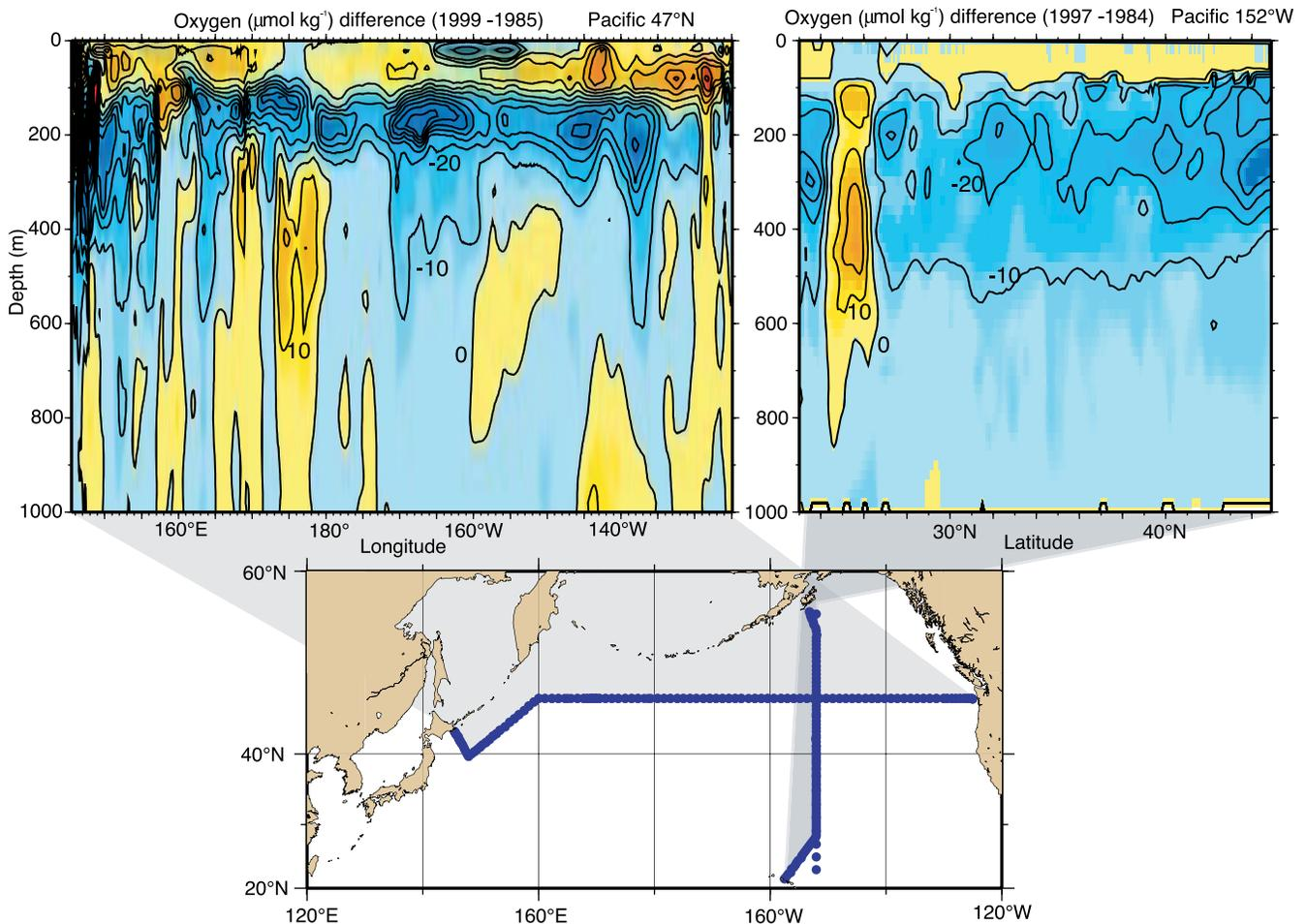
**Figure 5.12.** Changes in oxygen concentration ( $\mu\text{mol kg}^{-1}$ ) along two sections in the North Pacific (see map, bottom panel). Top left panel: Difference (1999 minus 1985) along  $47^{\circ}\text{N}$ . Top right panel: Difference (1997 minus 1984) at  $152^{\circ}\text{W}$ . Blue colours indicate a decrease and yellow colours indicate an increase in oxygen over time. The differences were calculated using density as the vertical coordinate. After Deutsch et al. (2005).
