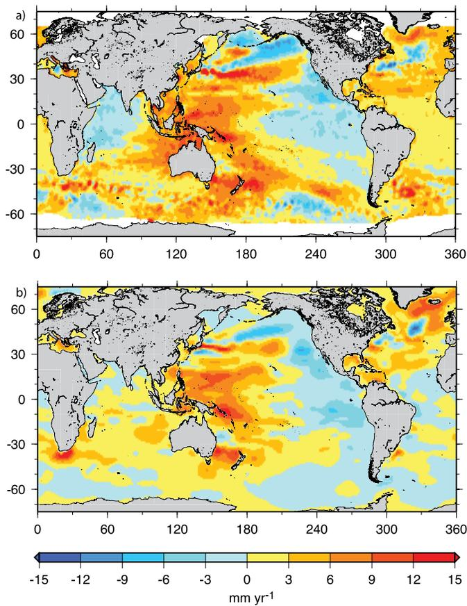
**Figure 5.15.** (a) Geographic distribution of short-term linear trends in mean sea level ( $\text{mm yr}^{-1}$ ) for 1993 to 2003 based on TOPEX/Poseidon satellite altimetry (updated from Cazenave and Nerem, 2004) and (b) geographic distribution of linear trends in thermal expansion ( $\text{mm yr}^{-1}$ ) for 1993 to 2003 (based on temperature data down to 700 m from Ishii et al., 2006).
