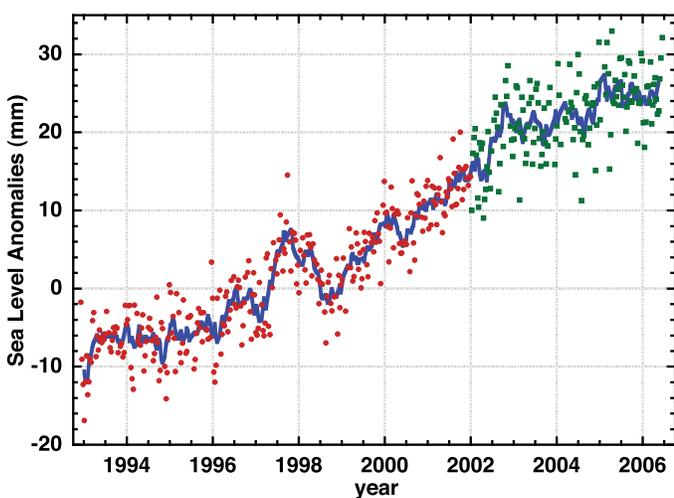
**Figure 5.14.** Variations in global mean sea level (difference to the mean 1993 to mid-2001) computed from satellite altimetry from January 1993 to October 2005, averaged over  $65^{\circ}\text{S}$  to  $65^{\circ}\text{N}$ . Dots are 10-day estimates (from the TOPEX/Poseidon satellite in red and from the Jason satellite in green). The blue solid curve corresponds to 60-day smoothing. Updated from Cazenave and Nerem (2004) and Leuliette et al. (2004).
