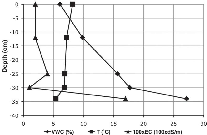
**Figure 4.** Plot showing volumetric water content (VWC), temperature (T), and electrical conductivity (EC) with depth in a water track soil column.
