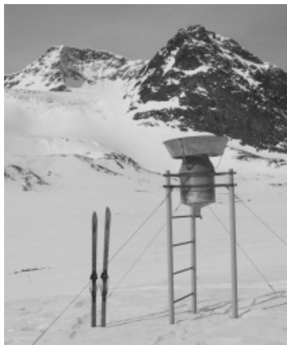
Figure 5. Totalisator collecting annual snow and rain precipitation. Isfallsgläciären in the background (Photo Mart Nyman).
