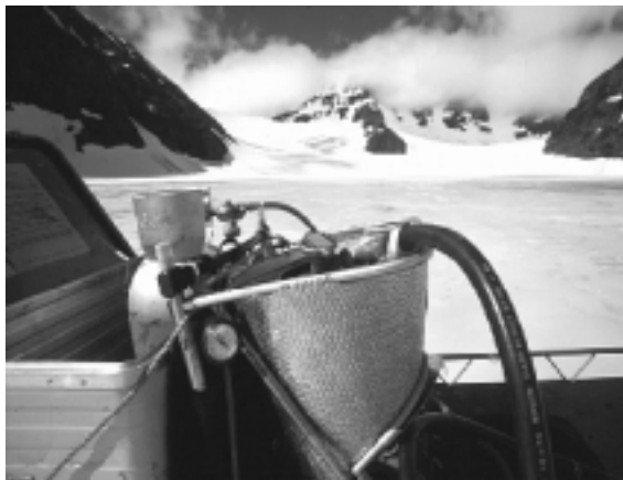
Figure 2. Images from field site showing a) the steam-pressure drill used to drill the 210 m of ice required for 42 stakes, and b) GPS surveying with Trimble's system 4000.
