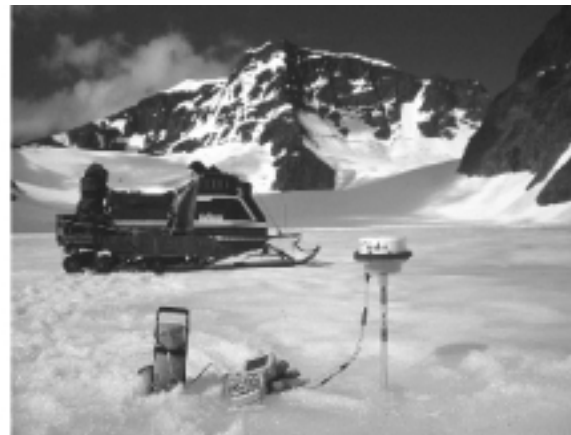
Figure 2. Images from field site showing a) the steam-pressure drill used to drill the 210 m of ice required for 42 stakes, and b) GPS surveying with Trimble's system 4000.
