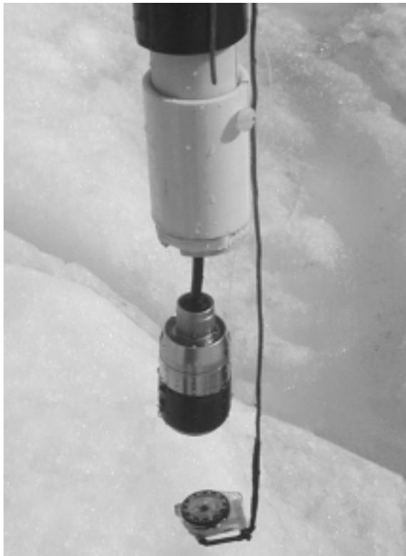
Figure 2. Borehole video camera with attached compass.
