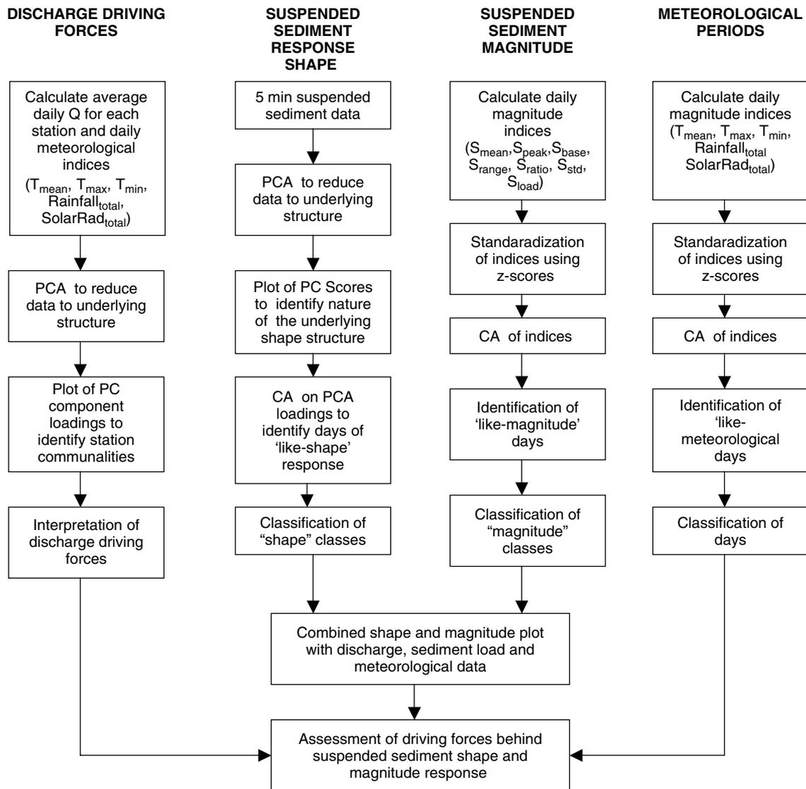
Figure 3. Flow chart detailing the classification procedures used to extract the suspended sediment transfer patterns: Q, discharge; T, temperature ( $^{\circ}\text{C}$ ); S, suspended sediment concentration (mg/L); Rainfall (mm); SolarRad(iation) (MW/day)
