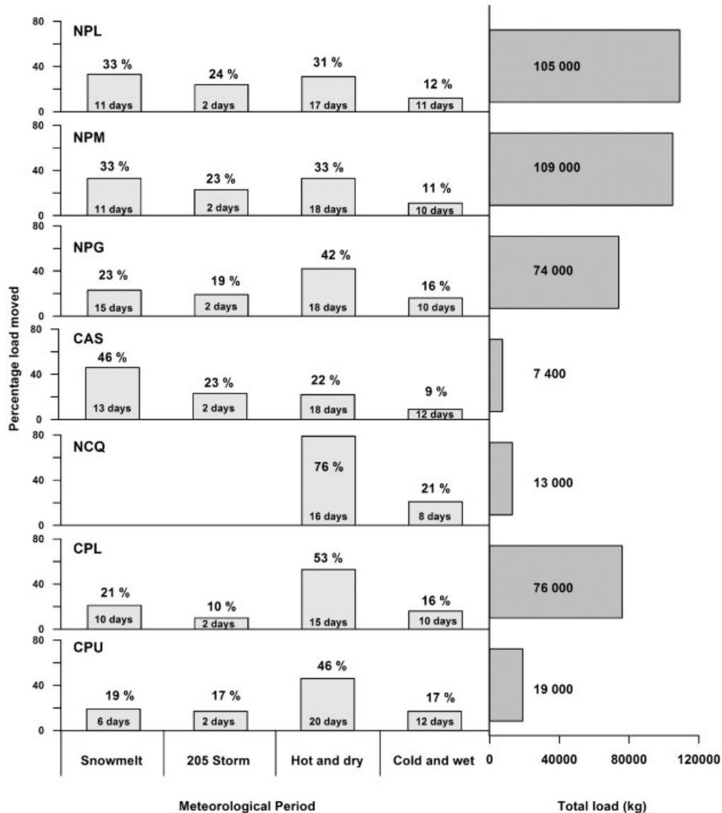
Figure 9. Suspended sediment load patterns for individual gauging stations during each meteorological period. Note that only loads from full hydrological days were used
