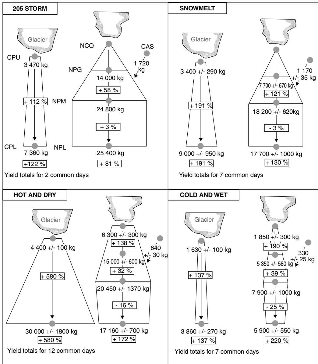
Figure 10. Proportional figures of suspended sediment yield from representative common days for each meteorological period. Note the significant spatial variability in yield response as determined by different catchment locations and meteorological conditions. Filled circles represent the gauging stations shown in Figure 1. Central Proglacial Middle and North gauging stations are not shown
