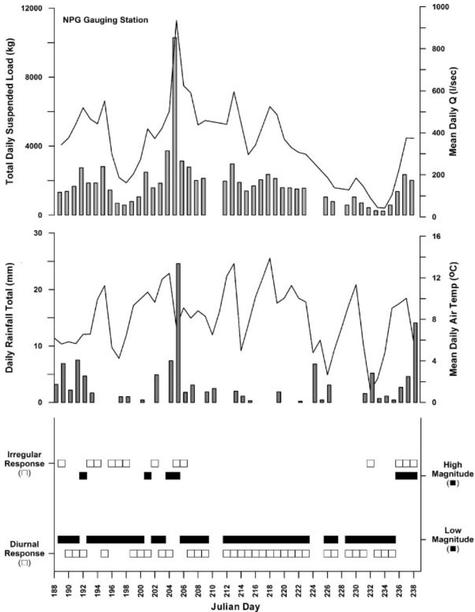
Figure 7. Example of a composite daily suspended sediment 'shape' and 'magnitude' response graph used to determine whether differences in catchment and meteorological conditions generated distinctive responses at each gauging station. The graph shown is for the North Proglacial gauging site where suspended sediment transfer patterns were dominated by a low 'magnitude' diurnal pattern. 'High' magnitude events were associated with rainfall events
