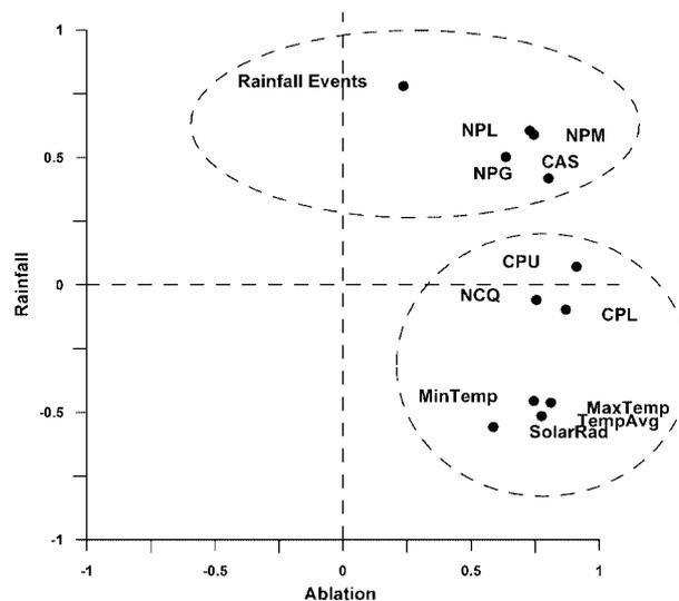
Figure 5. Principal component loadings for meteorological variables and all stations for the ablation season of 2000. Station groupings indicate the relative dominance of ablation and/or precipitation on discharge generation for each gauging station. The 'Ablation' and 'Rainfall' PC's explain 55% and 22%, respectively, of the total variance in the PCA. Letter codes refer to individual gauging stations (see Figure 1)
