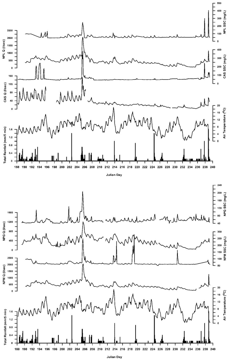
Figure 4. Raw 5-min data series of discharge (l/sec) and suspended sediment concentration (mg/L) used in the PCA and CA analyses for all gauging stations. Rainfall (mm/5 min) and air temperature ( $^{\circ}$ C) have been included for comparison. Letter codes on the axes refer to individual gauging stations (see Figure 1)
