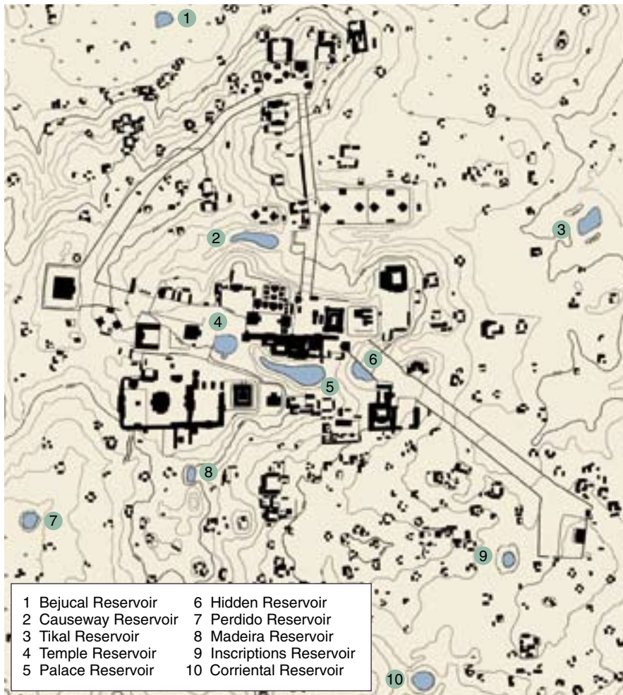
Figure 2. Maya cities commonly depended on artificial reservoirs to provide a year-round source of water. The residents of Tikal, for example, constructed several reservoirs (blue) near the city center, enough to provide 10,000 people with drinking water for 18 months. (Adapted from map of Carr and Hazard 1961, courtesy of the University of Pennsylvania Museum.)
